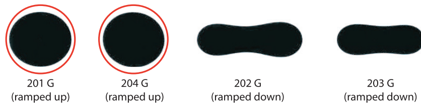
Figure 6. Equilibrium patterns of a magnetic liquid in a Hele–Shaw cell for (approximately) the same magnetic field values differ depending on whether the field is ramped up or down. The patterns are (nearly) circular when the field is ramped up and elongated when the field is ramped down. This clearly demonstrates hysteresis and a double energy minimum. The final magnetic field values correspond to bond numbers between 1.36 and 1.38.
